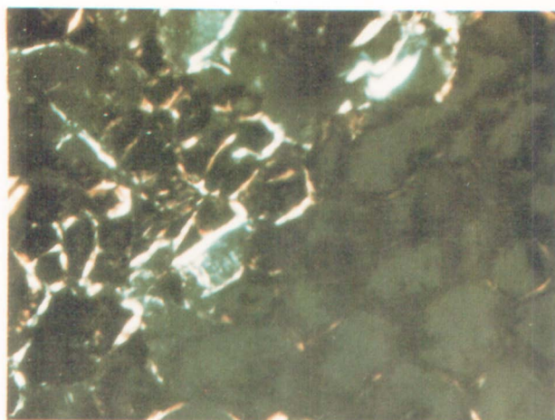
Figure 5b. Same view as 5a except under cross-polarized light to show birefringent ingredients. The less stained walls are the most birefringent.
